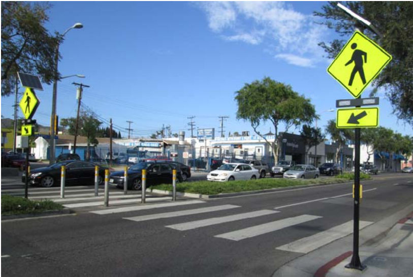
A typical RRFB
